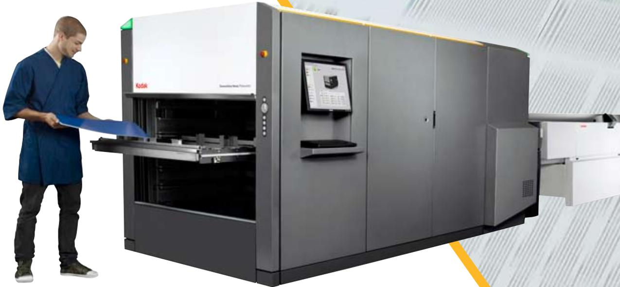
Multiple plate cassettes with automated loading allow you to run continuously for longer.
